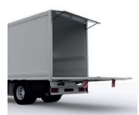
Truck with tail lift (hydraulic platform)
