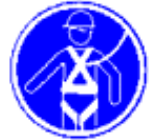
Personal fall protection is required when working at more than 3.5 m. and recommended as of 2 m.
